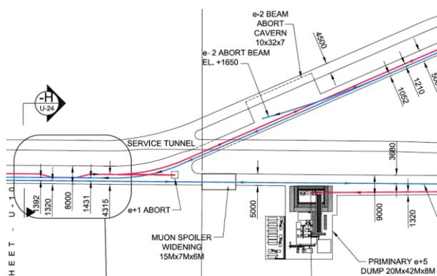
Figure 2: Detail of the Americas region tunnel design [2]; the same region as in Fig. 1 is depicted. The beam-lines are drawn directly from imported lattice data.
