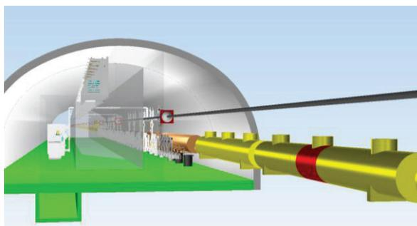
Figure 3: View of the conceptual lattice visualization (foreground) together with a detailed tunnel design for the sites with mountainous topography ("Kamaboko" shape, in the background).
