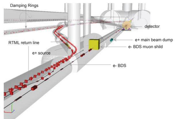
Figure 1: Example for design integration: the region where the transfer-tunnel branches off from the electron main tunnel towards the damping rings is shown. The European tunnel is shown together with a visualisation of the electron RTML and BDS and the positron-source beamlines. The transfer-tunnel geometry was changed in the central-region integration process in order to avoid the region around the positron main dump and the electron BDS muon shield.
