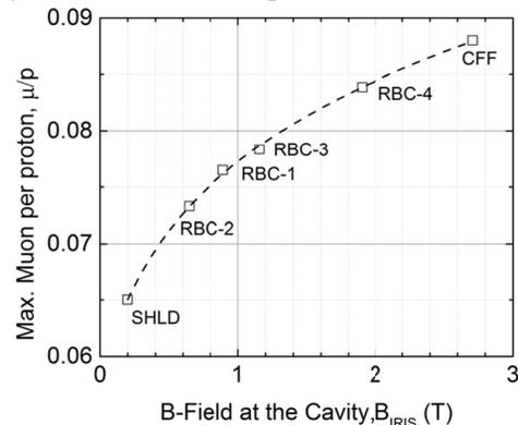
Figure 4: Lattice performance versus the magnetic field on the cavity iris. Higher field on the iris implies also better performance.
