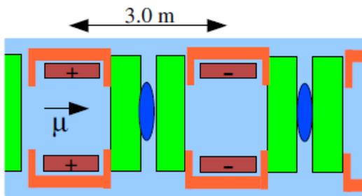
Figure 3: Shielded coil system. The lattice period is 3 m and each cell has two cavities (green) and one LiH absorber (blue).
