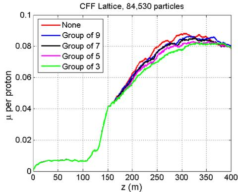
Figure 2: Performance of the lattice shown in Fig. 1(a) as a function of the number of cavities before the “empty” cell.
