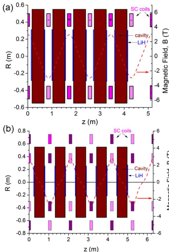
Figure 1: Two different cooling schemes for a Neutrino Factory: (a) A conventional flip focusing channel; (b) A radial bucked coil lattice.
