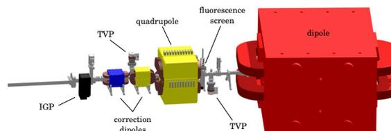
Figure 4: The second section of the beamline. The vacuum is maintained by two TVPs and one IGP. Two correction dipoles—one for each plane—are followed by the second, soled quadrupole with a maximum field gradient of 40 T/m. Once again, a fluorescence screen is installed behind it. The dipole bending magnet comes next, whose task consists in guiding the beam to the test area.
