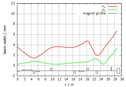
Figure 7: Simulation of the beam width development for an elliptic beam with radii of 5 mm and 2 mm, respectively at the test area.
