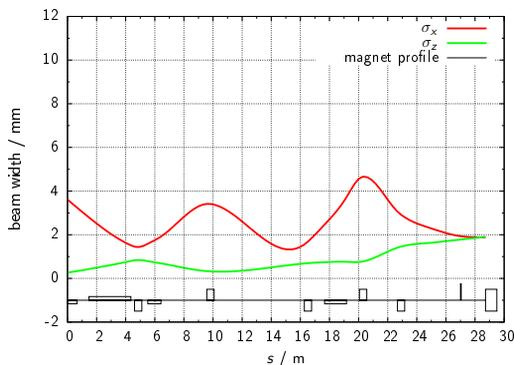
Figure 6: Simulation of the beam width development for a round beam of 2 mm radius at the test area.
