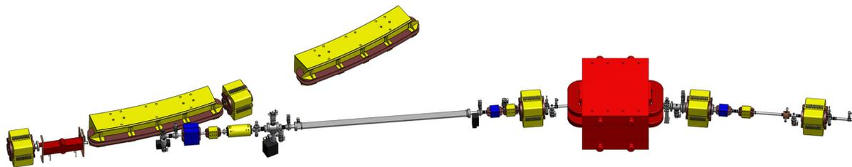
Figure 2: The layout of the beamline. On the left side, the ELSA ring with two quadrupoles and two dipoles as well as the main extraction septum can be seen. The new beamline branches off to the right.
