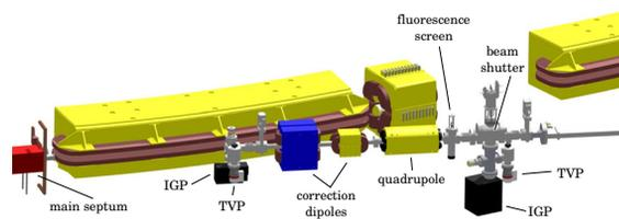
Figure 3: The first section of the beamline. The vacuum is ensured by two IGPs and two TVPs each at the beginning and at the end. A horizontal correction dipole is followed by a vertical one. Hereafter, the first quadrupole—featuring a maximum field gradient of 8 T/m—with a fluorescence screen behind it is installed. A beam shutter prevents electrons and synchrotron radiation to reach the test area.
