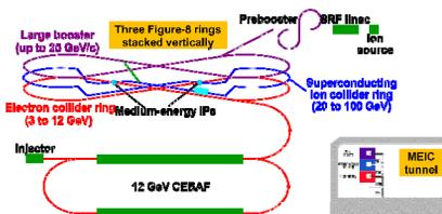
Figure 1: A schematic drawing of the MEIC design concept. The inserted picture on the low right corner shows a cross section of the envisioned MEIC tunnel.
