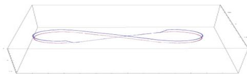
Figure 2: A 3D layout of the LEIC electron (red) and ion (blue) collider rings. The ion beam takes a vertical excursion to collide with electron beam.
