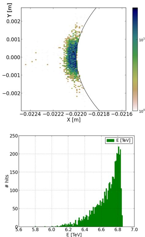
Figure 5: Transverse (top) and energy (bottom) distribution of the losses corresponding in the first peak in the dispersion suppressor right of IR7:  $20270 \text{ m} < s < 20350 \text{ m}$ . The black circle represents the aperture of the arc. The highest energy for a lost particle is 6.86 TeV, giving  $\delta p/p = -0.02$ .
