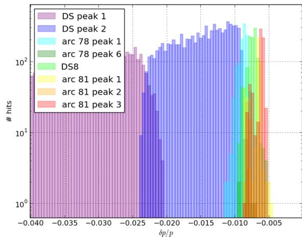
Figure 6: Distributions of the  $\delta p/p$  of the particles lost in the main peaks downstream IR7, grouped by peak. The names are arbitrary. There is a clear limit of  $\delta p/p$  under which the particles are lost.
