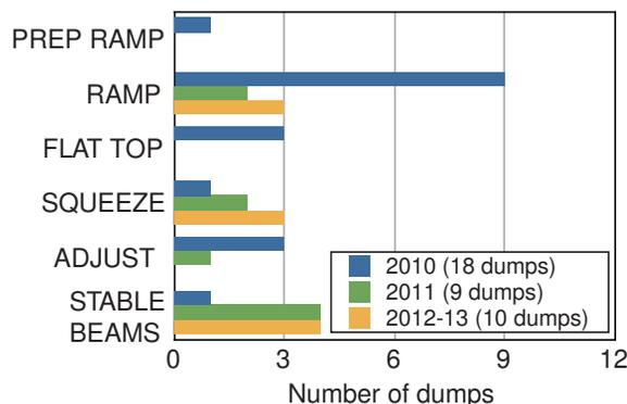
Figure 1: Number of dumps triggered by the collimation system above injection energy, listed per machine mode.
