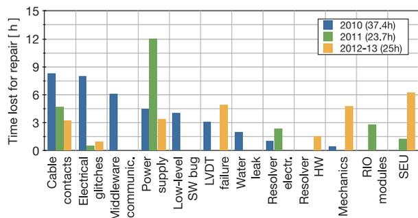
Figure 5: Machine down-time caused by collimator faults. Only failures that could not be recovered in the shadow of other systems faults are listed. Beam times required to re-validate the system after failures is not included.
