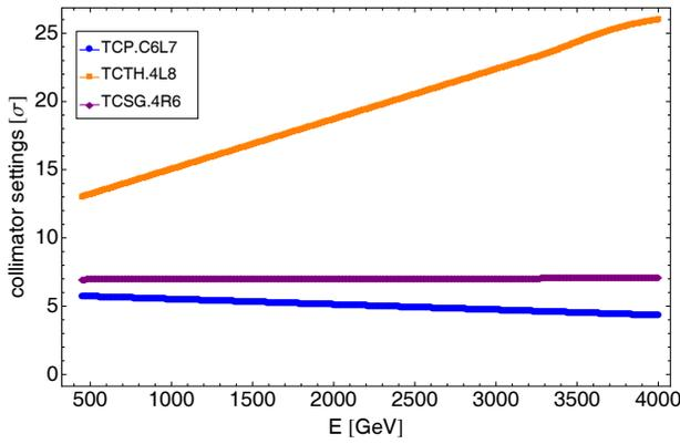
Figure 1: Collimator settings during the energy ramp.
