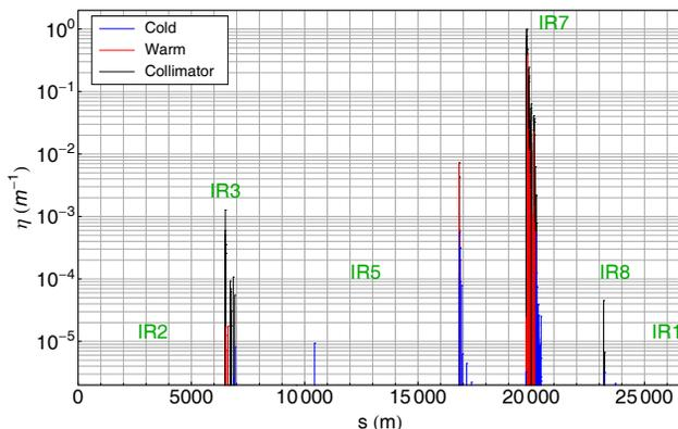
Figure 4: Measured horizontal loss map at 2 TeV.
