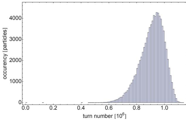
Figure 3: Histogram of the number of turns after that the first hit of the IR3 TCP jaw occurs.
