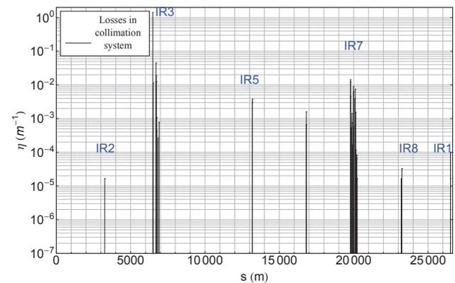
Figure 2: Beam loss map from SixTrack simulation at 7 TeV with synchrotron radiation effect.
