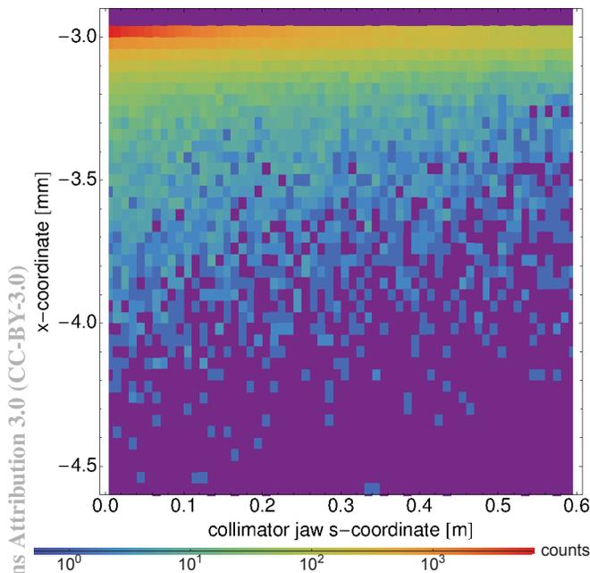
Figure 4: Density plot of particle impact parameter as function of longitudinal coordinate in IR3 TCP right jaw.
