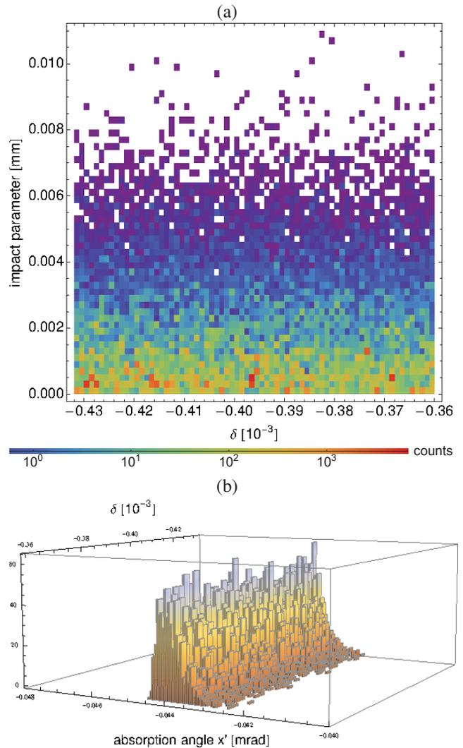
Figure 5: Correlation between the initial energy offset  $\delta$  and the impact parameter (a), the impact angle (b).
