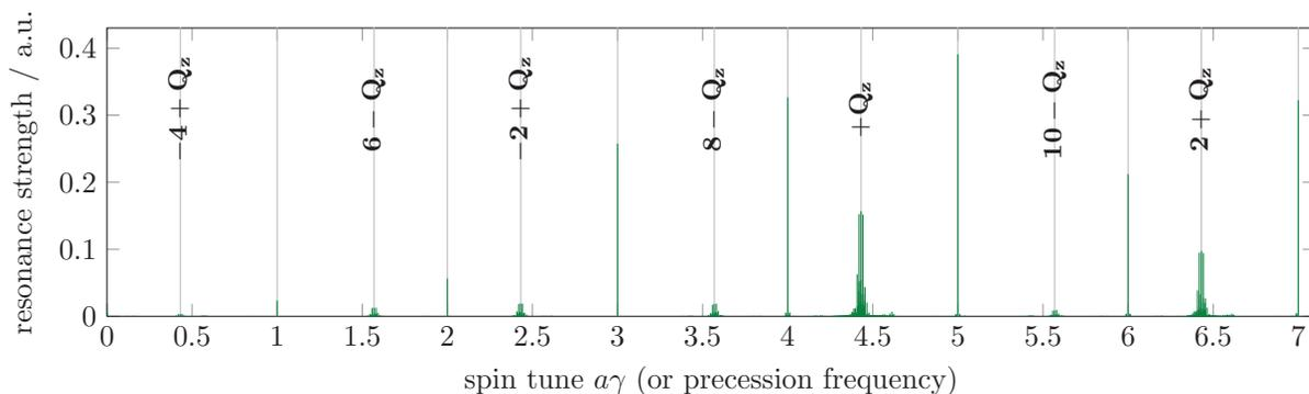
Figure 4: First results for resonance strengths in the ELSA stretcher ring predicted with POLE based on a MAD-X particle tracking for emittance 500 nmrad, vertical tune  $Q_z = 4.431$  and periodicity  $P = 2$
