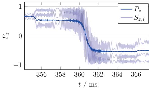
Figure 2: Simulated vertical polarization with synchrotron side-bands during crossing of integer resonance  $a\gamma = 6$
