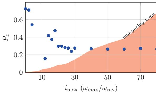
Figure 1: Simulated vertical polarization after crossing of integer resonance  $a\gamma = 3$  as a function of the maximum considered frequency of the magnetic field spectrum
