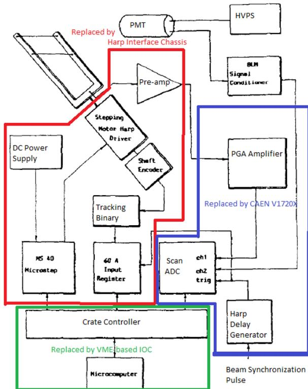
Figure 1: A diagrammatic sample of hardware reduction between the existing and modernized systems.
