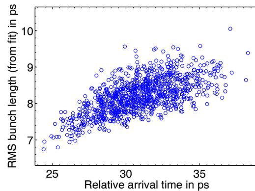
Figure 4: Scatter plot showing a correlation between the RMS bunch lengths retrieved by Gaussian fits for 1000 consecutive single shot EOSD measurements and their arrival time relative to the laser pulse.
