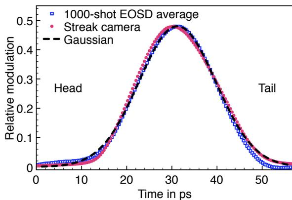
Figure 3: Comparison of the bunch profile recorded with EOSD by averaging over 1000 aligned single-shot measurements and an averaged bunch profile (average over 100 images, aligned slice-wise) recorded by our Hamamatsu streak camera simultaneously. In addition a Gaussian profile is plotted as reference. The data sets agree very well in bunch length, but the profile recorded with the streak camera shows a small asymmetry at the peak.
