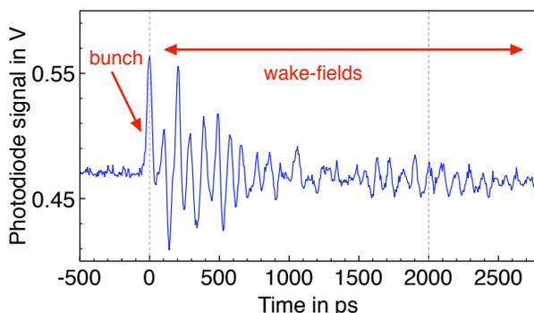
Figure 1: EOS measurement of the electric field induced birefringence inside the GaP crystal from a passing electron bunch.
