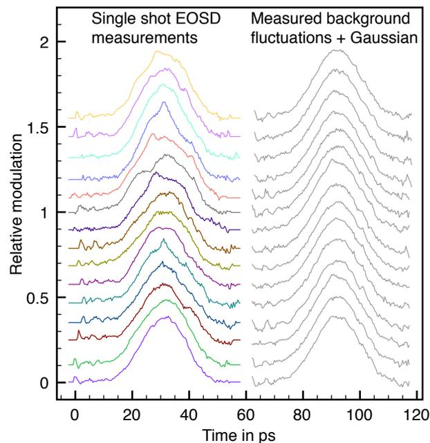
Figure 2: Left: 15 consecutive single shot EOSD measurements recorded at about 3 Hz. For better visibility, they have been displaced vertically and aligned horizontally to correct for any time of arrival fluctuations. Right: 15 unmodulated spectra divided by the same average modulated spectra as the measurement data on the left and added to a Gaussian to illustrate the influence of background fluctuations and noise for comparison (see main text).
