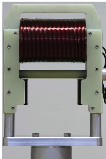
Figure 2: New vertical corrector magnet.
