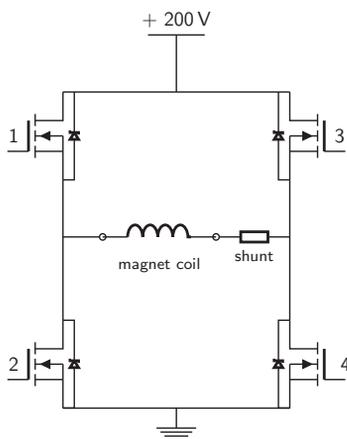
Figure 3: H bridge: Four NMOS transistors STY140NS10 are arranged like the four legs of the letter H, the magnet coil together with a shunt resistor taking the place of the horizontal bar.
