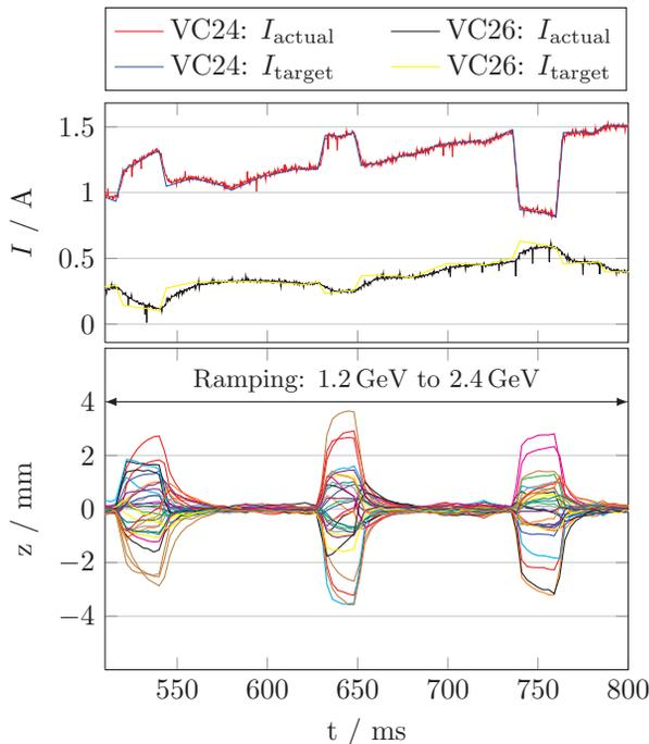
Figure 4: Status of the corrector system: In the top part the target and actual currents of two exemplary chosen vertical correctors are shown. These are the currents for vertical orbit correction superposed with additional currents for harmonic correction at three well-chosen energies. In the lower part the development over time of all 32 vertical beam positions is plotted.
