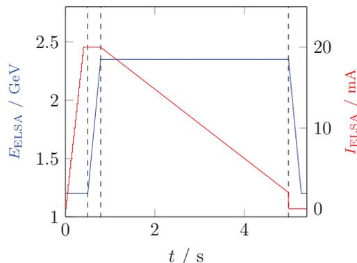
Figure 1: For the first 500 ms several injections are accumulated, followed by a fast energy ramp (4 GeV/s). For the next four seconds the circulating current is continuously extracted by slow resonance extraction. After that the energy is ramped down and a new injection is prepared.
