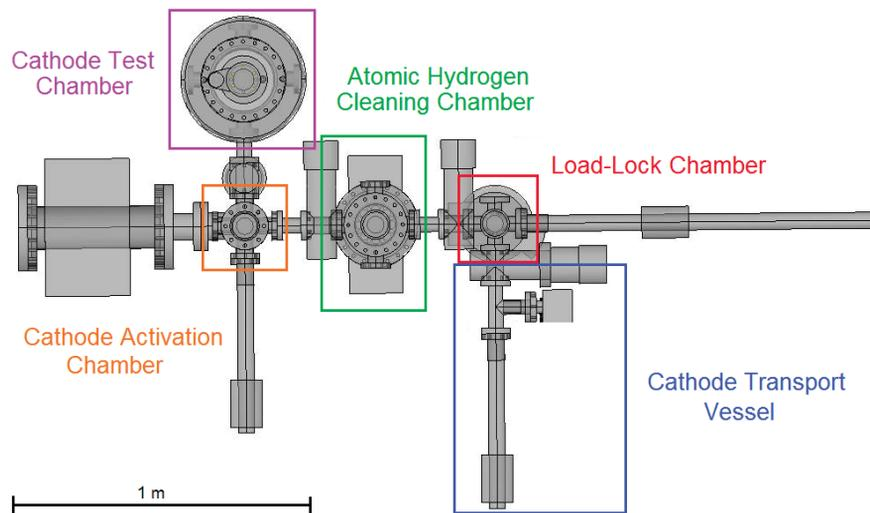
Figure 4: First concept of the new atomic-hydrogen cleaning system.
