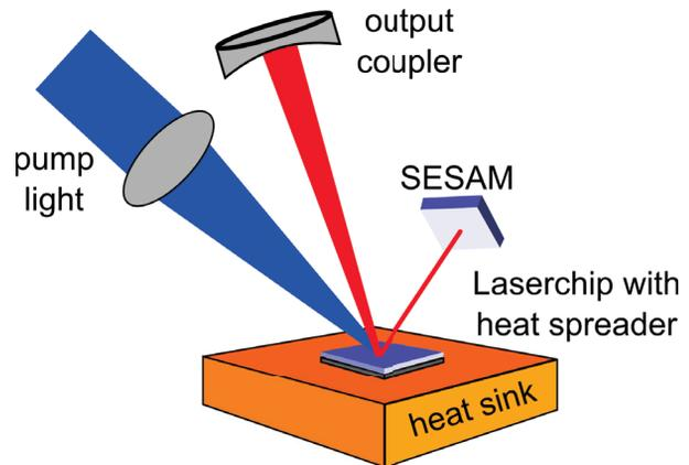
Figure 3: Principle configuration of a VECSEL.
