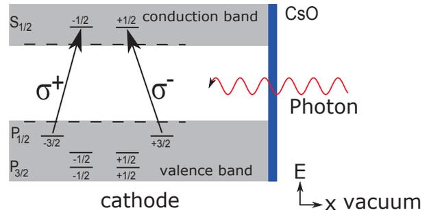
Figure 1: Principle of generating spin-polarized electrons with strained-superlattice-GaAs photo-cathodes.
