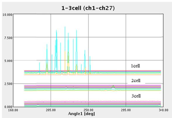
Figure 6: Temperature mapping results during self-pulsing at Eacc = 22.7 MV/m, obtained at first vertical test of ERL 9-cell #4 cavity.
