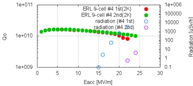
Figure 5: Vertical test results for ERL 9-cell #4 cavity. Left and right axes show  $Q_0$  and radiation dose, respectively.
