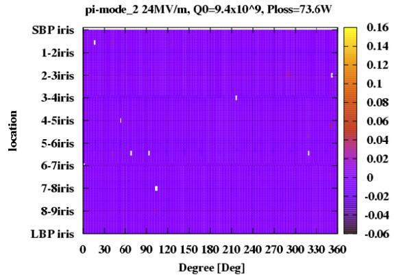
Figure 7: X-ray mapping results at Eacc = 24 MV/m, obtained at second vertical test for ERL 9-cell #4 cavity.
