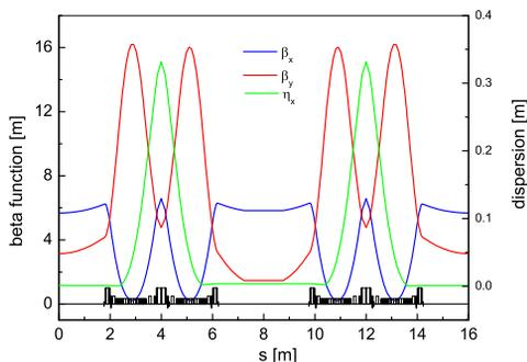
Figure 1: Two achromats with a 3.5 T SCW inserted in between.
