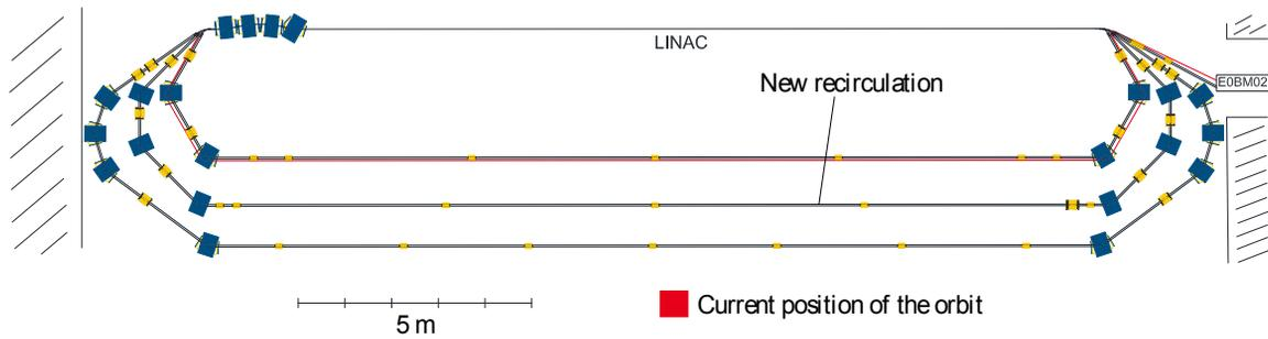
Figure 1: Sketch of the S-DALINAC with three recirculations, without the injector part.
