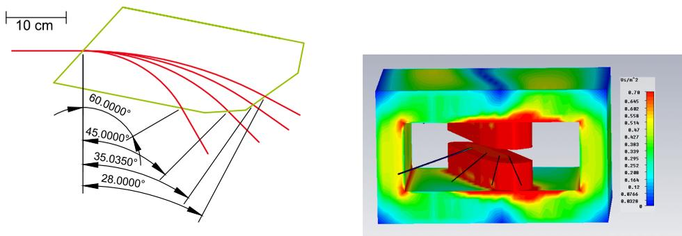
(a) Sketch of the new separation dipole with indicated orbits and bending angles (top view). The green lines enclose the area of ideal magnetic field, the red lines indicate the orbits of the four beams. The bending angles are given.
