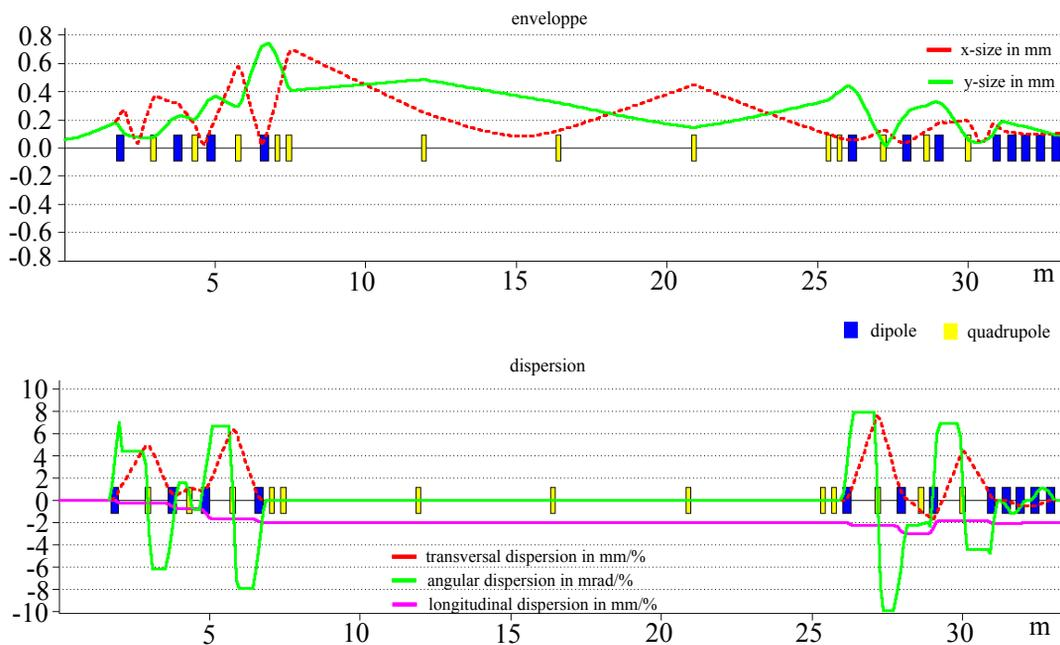
Figure 3: Beam dynamics of the new recirculation under the lattice assumed so far.
