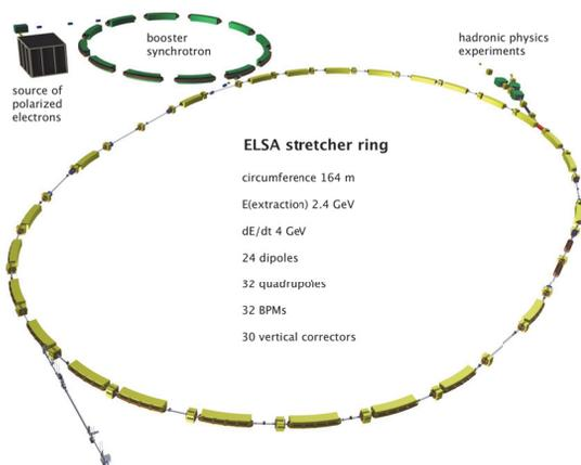
Figure 1: Overview of ELSA. The BPMs measure the orbit of the electrons at the point, where they are located.
