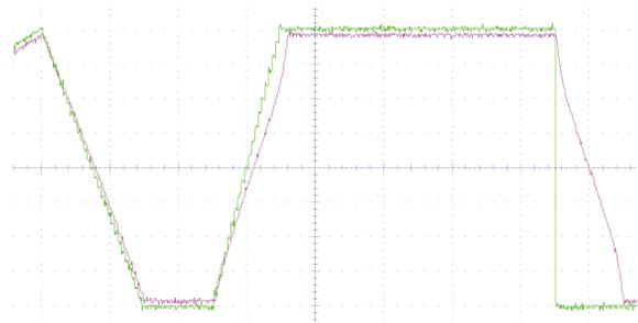
Figure 5: Scope shot of desired (green) and actual (pink) values of the current in a new coil, measured in a laboratory setup. The scales are 2 A/div vertically and 20 ms horizontally. The small deviations seen in the flat regions don't matter, because the magnet current is set by the control system in relation to the beam position.
