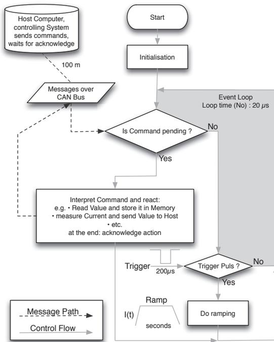
Figure 4: Flow diagram of the firmware operation.
