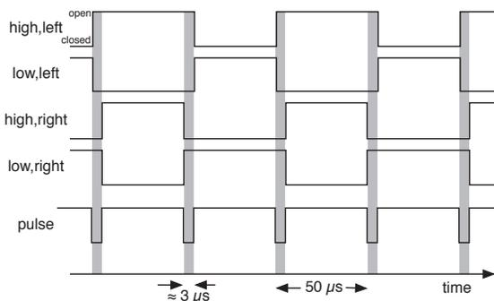
Figure 3: Timing diagram for the bridge.
