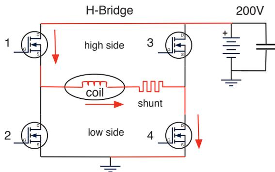
Figure 2a: Schematic of the bridge, current is injected.
