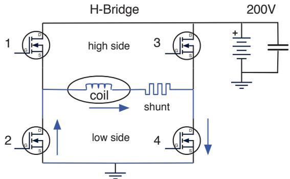
Figure 2b: Schematic of the bridge, current flows freely.
