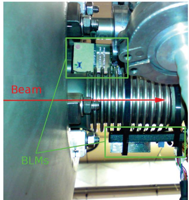
Figure 3: Beam loss monitors mounted directly onto the beam pipe in a narrow spot behind the injector cryostat.
