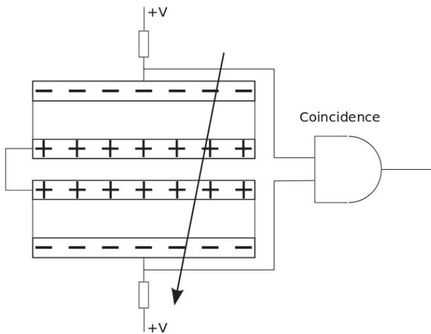
Figure 2: Operating principle of semiconductor beam loss monitors based on diodes.
