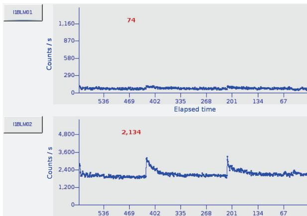
Figure 4: Electric charging effects can be observed directly through rising count rates of the beam loss monitors. The upper graph corresponds to a BLM located 0.5 m off the beam pipe, the lower one corresponds to a BLM attached directly to the vacuum chamber.
