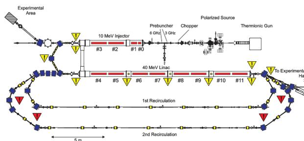
Figure 1: Floor plan of the S-DALINAC. Yellow triangles mark important locations for BLMs during beam optimization. Red triangles mark other potentially interesting positions for those monitors.
