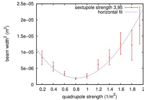
Figure 5: Quadrupole scan [3].
