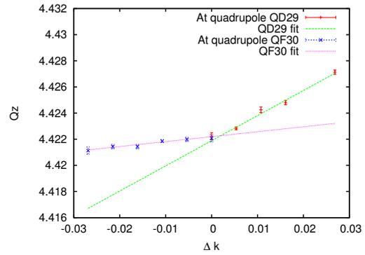
Figure 4: The vertical tune in dependence of the quadrupole strength. The corresponding linear fits are included as well.
