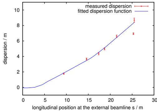
Figure 3: Dispersion at the external beamline.
