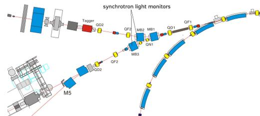
Figure 2: Synchrotron light monitors at the external beamline [3].
