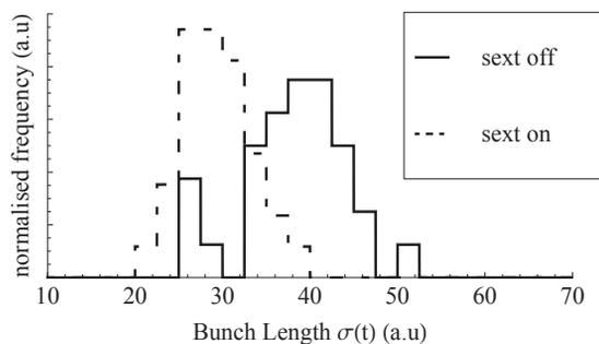
Figure 5: ALICE compressed bunch length measured by electro-optic technique, with the first sextupole in the first arc turned on and off. The horizontal scale is arbitrary units, an indicative scaling is 50 units/ps or 150 units/mm.
