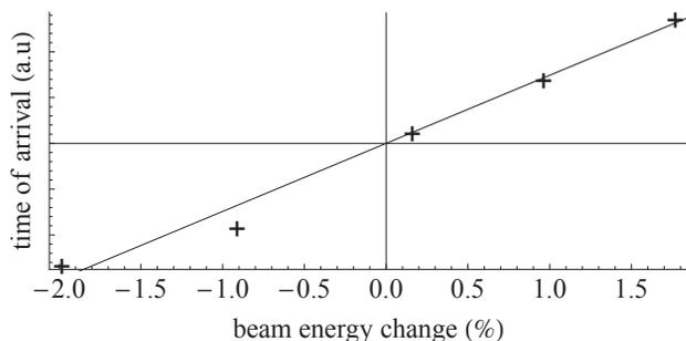
Figure 6: ALICE post-compression beam time of arrival (TOA) vs. beam energy. The TOA is displayed in arbitrary units but an indicative scaling is  $\sim 20$  ps for the full range of measurements shown here.
