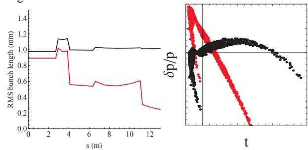
Figure 3: ELEGANT simulation of bunch length evolution in injector (left) for different longitudinal chirps at booster exit (right). The booster exit is located at  $s = 0$  m.
