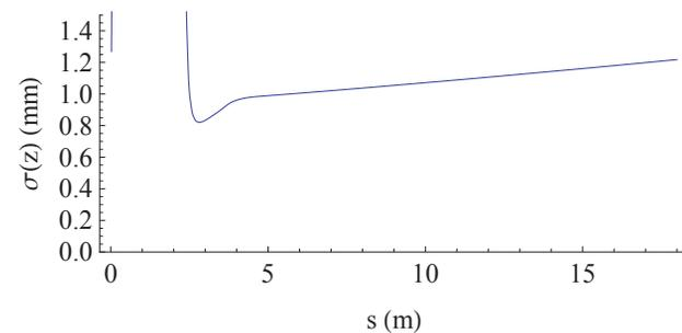
Figure 4: ASTRA simulation of bunch length evolution in a long drift space post-booster, for the larger chirped distribution in Fig 3. The booster exit is located at  $s \sim 5$  m.
