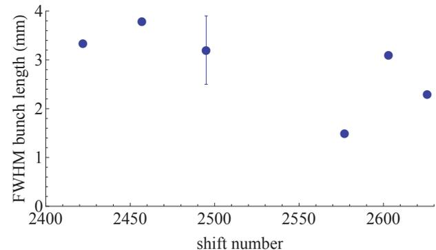
Figure 1: Injector bunch length measurements for a single machine set-up over a 5-month period. The injector bunch length is inferred at the exit of the first of the two booster cavities. The error was estimated on one measurement and is indicated by the error bar.
