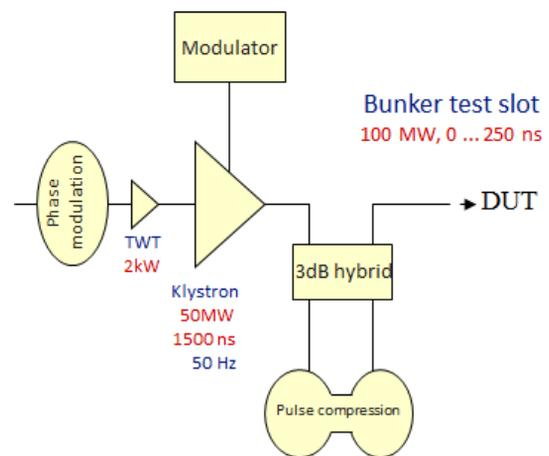
Figure 1: Layout of the CERN X-band power source.
