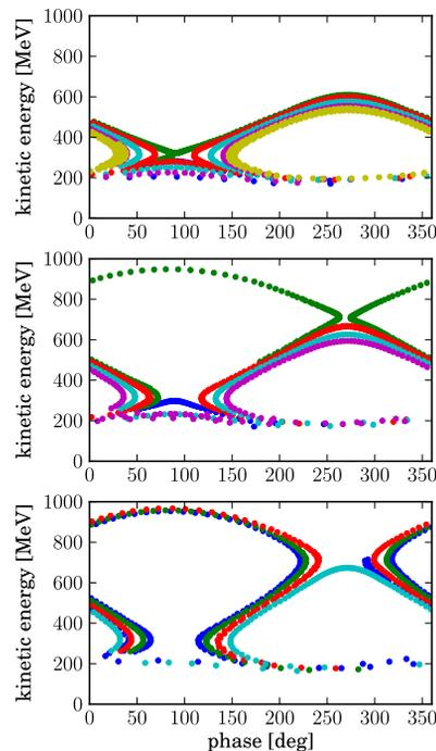
Figure 3: Longitudinal phase space (upper) with 10 MV/turn, an insufficient accelerating voltage to open a serpentine channel, (middle) with 12 MV/turn, a sufficient voltage for a serpentine channel less than  $1^\circ$  wide and (lower) with 15 MV/turn, for a serpentine channel with a  $20^\circ$  width.
