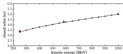
Figure 1: Variation of the closed orbit with energy established using OPAL (black), compared to the original COSY Infinity results (red markers).
