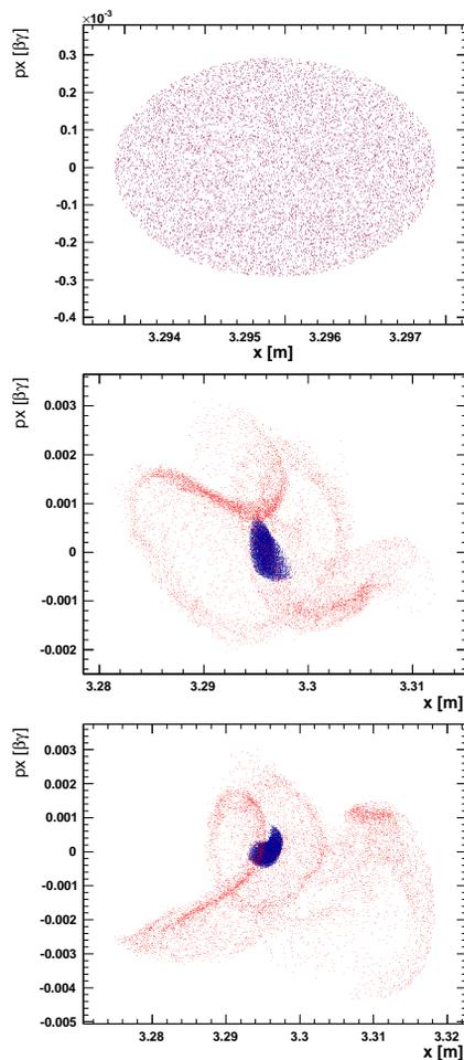
Figure 4: Example of tracking in OPAL with and without space charge for a 10 mA beam with  $10\pi$  mm mrad normalised transverse emittance.
