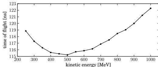
Figure 2: Variation of the time-of-flight per turn with energy established using OPAL.
