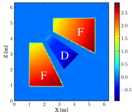
Figure 1: A field map of one quarter of the lattice showing the vertical magnetic field in Tesla. Magnetic field profiles are measured along the centre of the F and D magnets, shown in Fig. 2.
