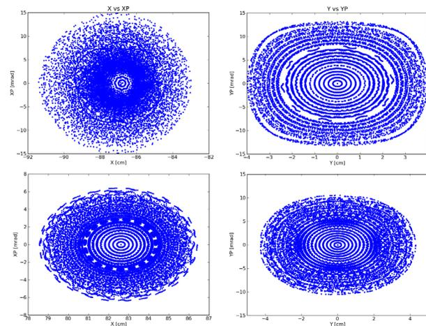
Figure 4: Phase space portraits for single particles tracked for 1000 turns starting with simultaneous horizontal and vertical offsets in steps of 2 mm at injection (upper) and extraction (lower) in the horizontal (left) and vertical (right) planes.
