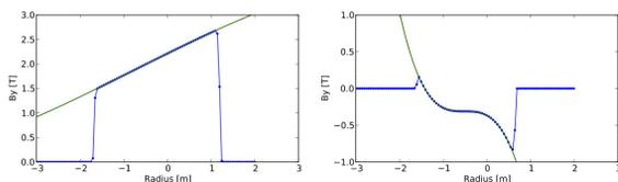
Figure 2: Radial field profile from field map (blue points) with polynomial fit (black line) for the F (left) and D (right) magnets, taken along the centre line of each magnet.
