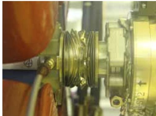
Figure 2: Deformation of the bellows with CT monitor installed on the endplate of the SDTL cavity.
