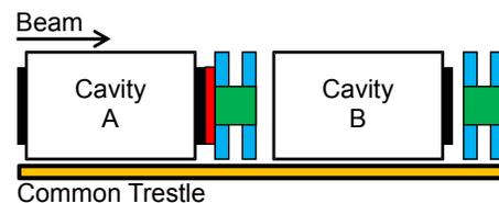
Figure 1: General Layout of the Beam Monitors in SDTL section. This describes a pair of SDTL cavities on a trestle, i. e. both A cavity (left) and B (right) cavity are installed together on the same trestle. The linac has 15 pairs of the SDTL cavities. Beam comes from the left side. Black boxes are FCT monitors, red one is SCT and green ones are BPMs.
