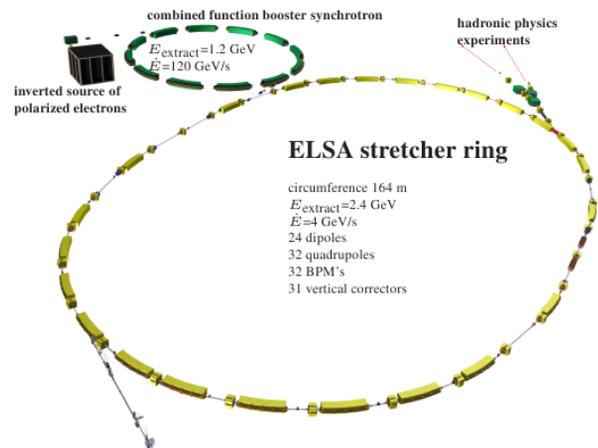
Figure 1: ELSA overview. Shown are the main parameters and components of the ELSA facility with regard to polarized operation performance.
