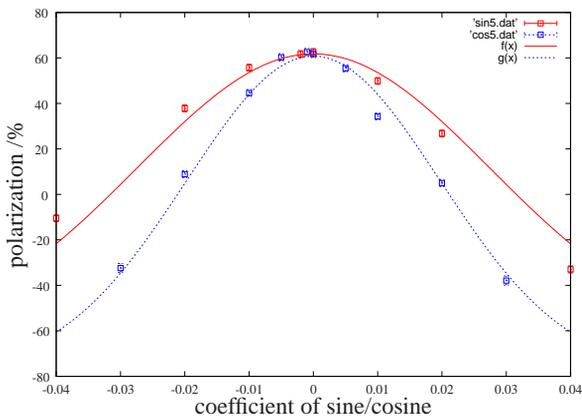
Figure 2: Empirical correction of the fifth integer spin-tune resonance. The measuring points of the sine part are red colored, the blue dots indicates the cosine part.
