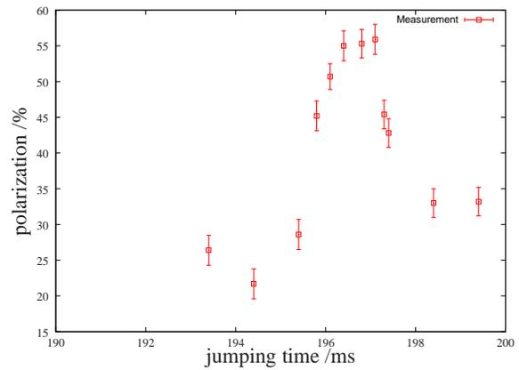
Figure 4: Performance of the tune jump when used at the resonance  $a\gamma = 0 + Q_z$ . The impact of the abruptly generated quadrupole field is a fast change of the optical tunes. Doing this accurately timed, a higher degree of polarization is preserved.
