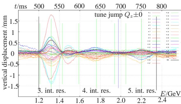
Figure 3: The vertical traces of the beam position monitors are shown (colored for each bpm and in black for RMS) during the energy ramp in the stretcher ring (1.2–2.4 GeV with 4 GeV/s). The correction for the integer resonances causes additional vertical displacements.
