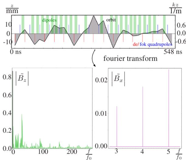
Figure 1: The upper figure shows a disturbed closed orbit, simulated with MAD-X, along a one-turn orbit length of the ELSA stretcher ring. The magnetic fields in the rest frame can be obtained by multiplying the color marked, magnetic field strengths by the vertical displacement. The lower figures show the spectra which result from the Fourier transformation.
