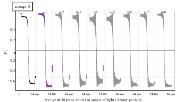
Figure 5: Solution of the numerical calculation of a spin-flip for a sample of eight particles including quasi-stochastic approach of synchrotron oscillations. On the left hand side, the polarization averaged for 50 particles is shown.
