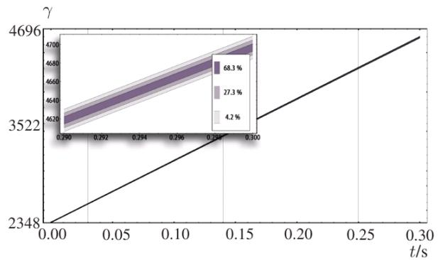
Figure 2: The figure shows the time dependency of the factor  $a\gamma(t)$ . The  $a\gamma$ -function is weighted according to the Gaussian shaped energy distribution of the beam. The color range inside the zoomed part of the figure represents the particle density in percent. The graph displays a typical situation at the ELSA stretcher ring. The energy of the electrons is ramped from 1.2 GeV up to 2.4 GeV within 0.3 seconds.
