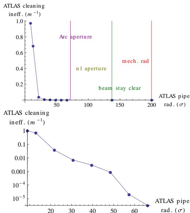
Figure 3: Maximum local cleaning inefficiency, normalized by TCT losses, in ATLAS (using 10 cm bins) for 7 TeV collision optics as a function of the beam pipe radius (top), shown with the design aperture for the upgrade, the guaranteed beam stay clear radius and the  $n1$  aperture [7]. The bottom plot shows the non-zero losses on a logarithmic scale.
