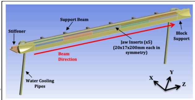
Figure 2: Lower symmetrical half of the collimator structure.
