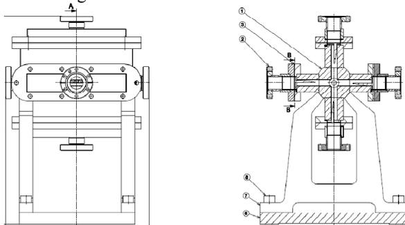
Figure 1: Design of the accelerating structure dedicated to the vacuum tests
