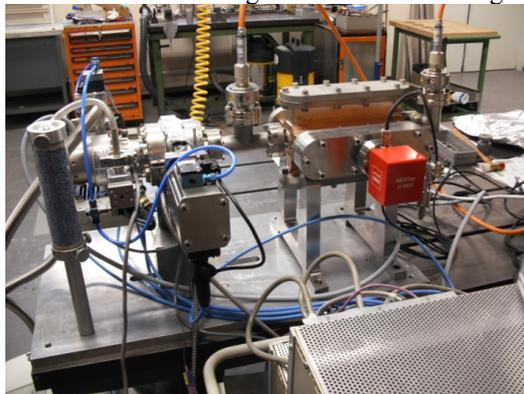
Figure 4: set-up with the NEG cartridge pump
