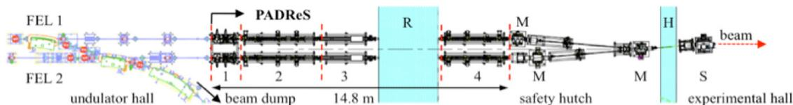
Figure 1: Layout of PADReS: 1, photon shutter and diagnostics; 2 and 4, differential pumping systems; 3, gas cell; M, mirrors vacuum chambers; S, energy spectrometer vac. chamber; R, radioprotection wall; H, safety hutch wall.
