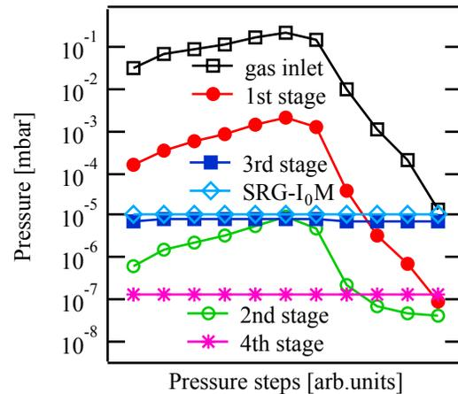
Figure 5: Effect of a pressure variation at the gas inlet on the differential pumping system when the  $I_0M$  is kept up to the nominal pressure.
