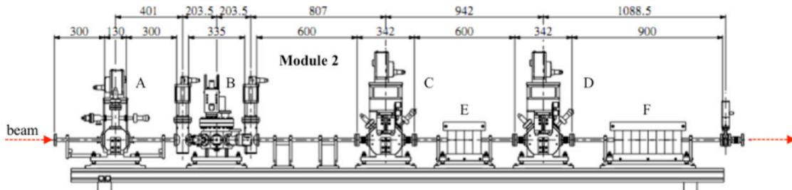
Figure 2: The 2<sup>nd</sup> module: A, interface to the ultra high vacuum chamber in module 1; B, intensity monitor; C, 1<sup>st</sup> beam stopper; D, 2<sup>nd</sup> BS; E and F, lead blocks around the connecting pipes.
