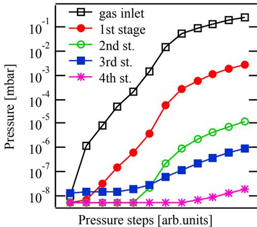
Figure 4: Effect of a pressure variation at the gas inlet on the differential pumping system.
