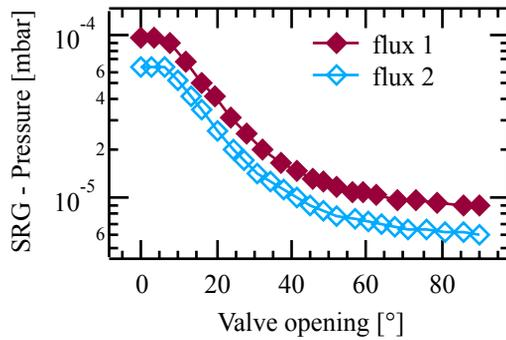
Figure 3: Pressure variation in the  $I_0M$  when a gas flux is injected and the butterfly valve angle is changed.
