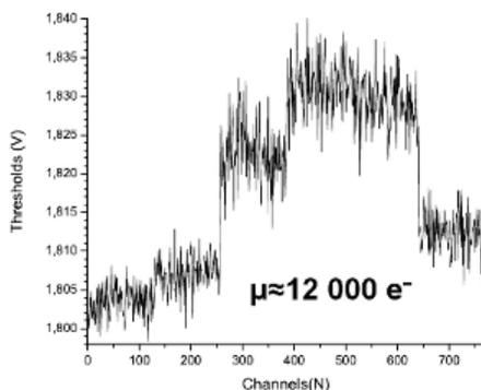
Figure 6: Threshold dispersion of the readout chips.
