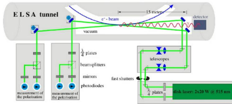
Figure 2: Set-up of the Compton polarimeter.
