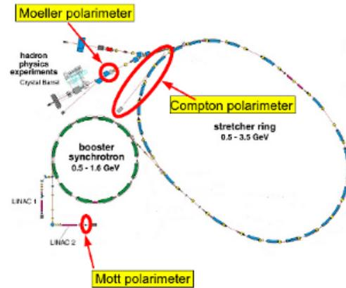
Figure 1: Electron stretcher facility ELSA with the positions of the Mott and Møller polarimeter as well as the proposed Compton polarimeter.
