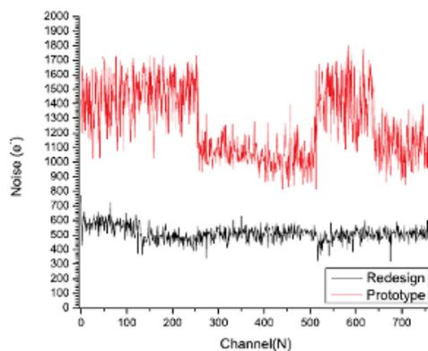
Figure 7: Comparison of noise levels of the counting chip in combination with the new/prototype detector board.
