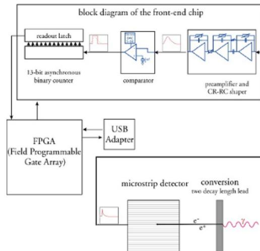
Figure 5: Schematic signal path for the detector system.
