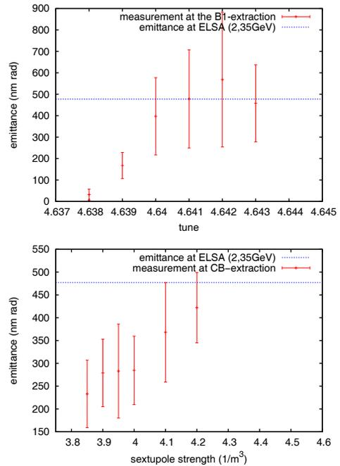
Figure 8: Dependence of emittance on extraction parameters. The blue line shows the equilibrium emittance at the stretcher ring.
