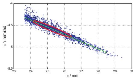
Figure 3: Coordinates in phase space after particle deflection into the extraction channel
