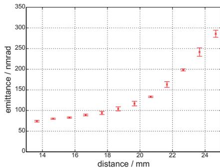
Figure 4: Emittance dependence on the distance of the septum to the design orbit
