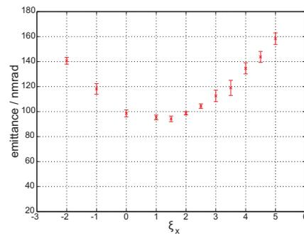
Figure 6: Emittance dependence on the horizontal chromaticity  $\xi_x$
