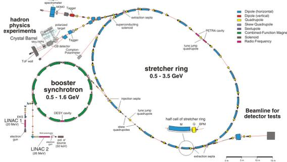
Figure 1: Electron Stretcher Facility ELSA
