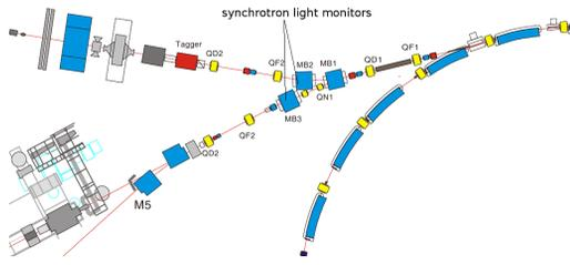
Figure 7: Synchrotron light monitors at the external beamline
