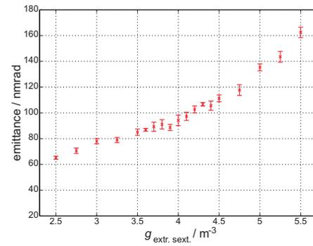
Figure 5: Emittance dependence on the strength of the extraction sextupole magnets
