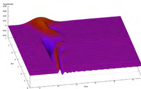
Figure 6: Response of the BPM to the rising bandwidth of the incoming Gaussian pulse.
