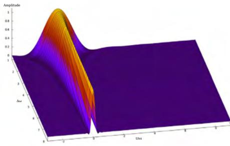
Figure 4: Gaussian pulses with rising bandwidth,  $\Delta\omega$ , transmitted through the monitor.
