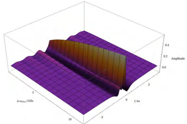
Figure 7:  $\mathcal{F}^{-1}(\text{BandPass} \times \mathcal{F}(\text{Gaussians}))$  for different bandwidths of the band pass,  $\Delta\omega_{\text{Filter}}$ .
