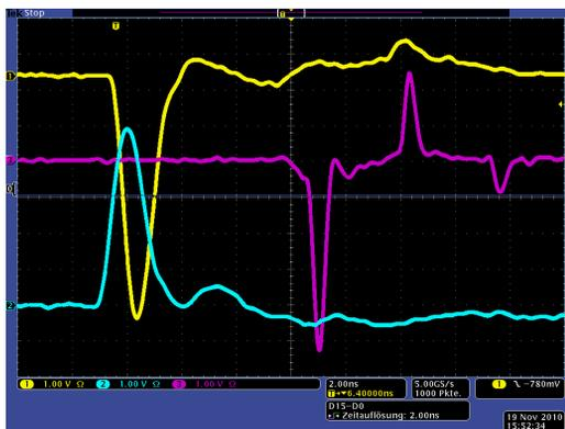
Figure 2: WCM1 (yellow), WCM2 (blue) and WCM3 signal (magenta) on an oscilloscope (for the locations see Figure 1). The absolute signal positions depend on the cable length, the signal polarities depend only on which way the connector is actually linked to the WCMs.
