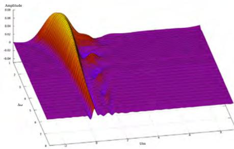
Figure 5: Response of the WCM to the rising bandwidth of the incoming Gaussian pulse.
