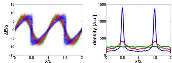
Figure 2: Phase space (left) of energy-modulated electrons and electron density (right) for different  $R_{56}$  values.
