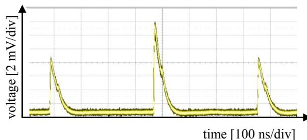
Figure 5: Oscilloscope image of the very first CHG signal at DELTA, showing three revolutions in single bunch mode. The central peak contains coherent contributions, whereas the others arise from spontaneous radiation.
