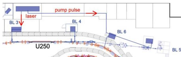
Figure 3: Northern part of the DELTA facility including the laser lab, the laser beamline BL3, the diagnostics beamline BL4 and the THz beamline BL6. An evacuated tube will send a fraction of each laser pulse (pump pulse) to the experimental station at BL5.
