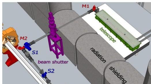
Figure 4: Model of the laser beamline BL3 showing the vacuum chamber with the telescope, beam shutter, mirror chambers M1, M2 and monitor screens S1, S2.
