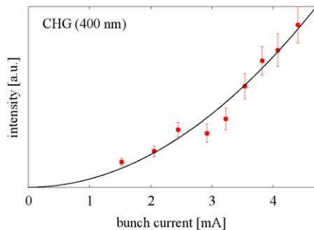
Figure 6: Dependence of the CHG signal (dots) on the bunch current fitted by a quadratic function (line).
