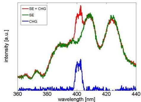
Figure 7: Spectrum of the optical klystron at DELTA with (red) and without (green) laser-induced modulation. The difference (blue) is the spectrum of the ultrashort CHG pulse.
