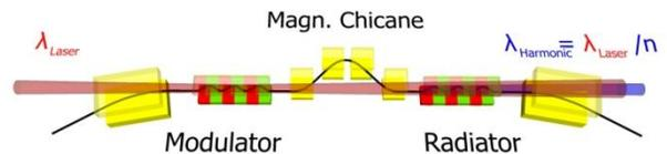
Figure 1: Schematic diagram of the CHG setup.
