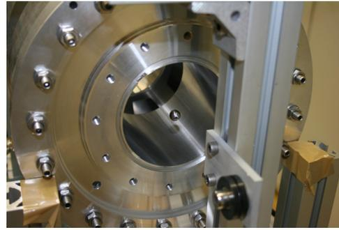
Figure 4: The experimental setup for measuring the electric field along the cavity axis using the bead ball perturbation method.
