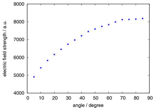
Figure 4: Calculation of the electric field strength on the beam axis of the stripline kicker in dependence of the opening angle of the striplines
