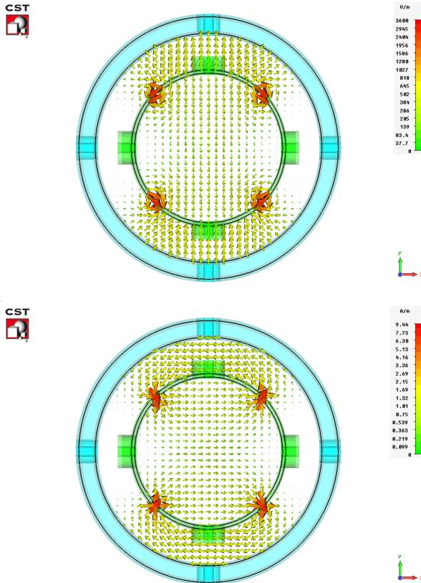
Figure 3: Electric (top) and magnetic (bottom) field distribution in the stripline kicker, when driving the upper and lower stripline
