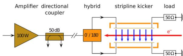
Figure 1: Driving scheme of the stripline kicker (vertical plane) using a broadband RF amplifier and a 0°/180° hybrid
