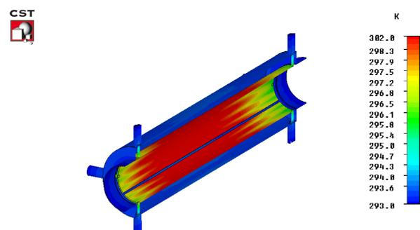
Figure 5: Heating up of the striplines due to resistive losses when driving the kicker with 200 W total power on four ports
