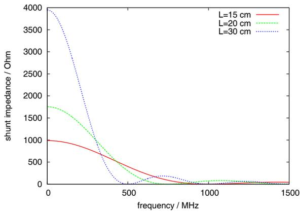
Figure 2: Shunt impedance of an ideal stripline kicker for different lengths of the striplines
