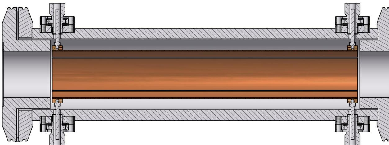
Figure 6: Cut through the final geometry of the new stripline kicker
