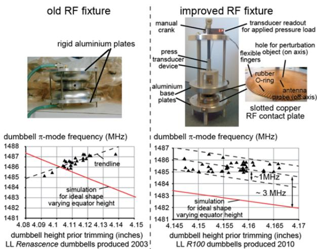
Figure 3: Prevalent frequency errors of past fabrication methods (left) cured by improved tooling (right).
