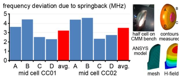
Figure 2: Frequency deviations of two deep-drawn cells from the ideal shape as measured at four different planes.
