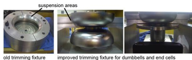
Figure 4: Old (left) and improved fixture (middle, right) for cell equator machining.
