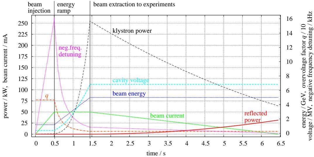
Figure 2: Accelerator cycle for a beam current of 50 mA up to an energy of 5 GeV using two SC cavities with a shunt impedance of  $R_s = 5 \cdot 10^{11} \Omega$  and an unloaded quality factor of  $Q_0 = 2 \cdot 10^9$ . Time dependence of cavity voltage and overvoltage factor, total klystron power as well as reflected power per cavity and negative frequency detuning per cavity.
