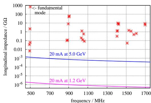
Figure 3: Longitudinal shunt impedances  $R_{\parallel}$  of monopole HOM and typical threshold impedances for longitudinal CBI at a beam current of  $20 \text{ mA}$  at ELSA.
