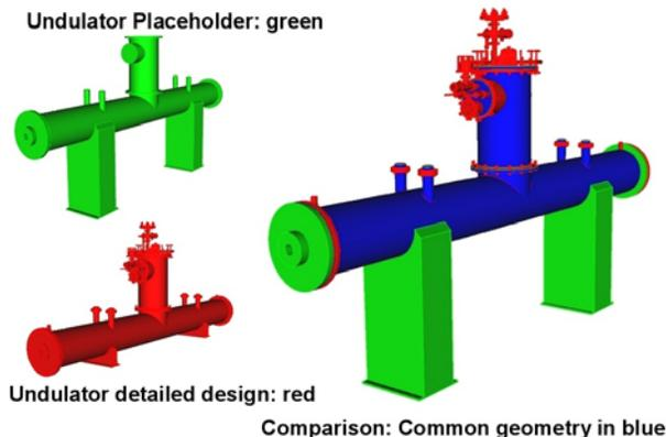
Figure 3: Comparison of placeholder and detailed design models
