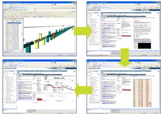
Figure 2: A single undulator cryomodule can be traced from its position within a 3D CAD model of the accelerator to the original lattice file stored in EDMS.
