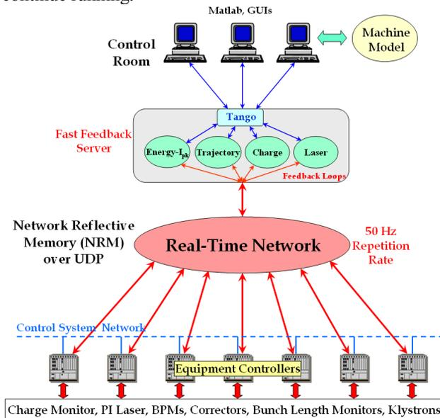
Figure 2: Fast feedback architecture.
