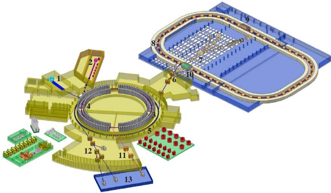
Figure 1: Scheme of NICA facility: 1 – light and polarized ion sources and “old” Alvarez-type linac; 2 – ESIS source and new RFQ linac; 3 – Synchrophasotron yoke; 4 – Booster; 5 – Nuclotron; 6 – beam transfer line; 7 – Nuclotron beam lines and fixed target experiments (to be dismantled); 8 – Collider; 9 – MPD; 10 – SPD; 11, 12 – transfer channels; 13 – new research area
