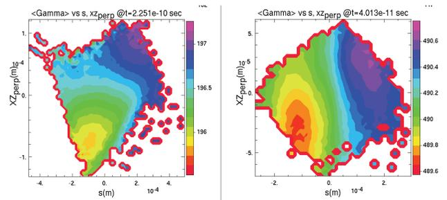
Figure 3: False color image showing  $\bar{\gamma}(s, r_\perp)$  at the simulation end for both the 100-MeV case of Figs. 1&2 (left plot) and a much shorter pulse ( $\sigma_z = 4.5 \mu\text{m}$  at 250-MeV traversing a 0.5-m long dipole with 26.7 m radius of curvature. Negative (positive) values of  $r_\perp$  correspond to particles whose transverse position (presuming laminar flow) was on the outer (inner) portion of the arc.
