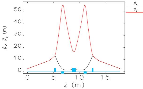
Figure 4:  $\beta$ -functions across symmetric insertion between two identical solenoids.
