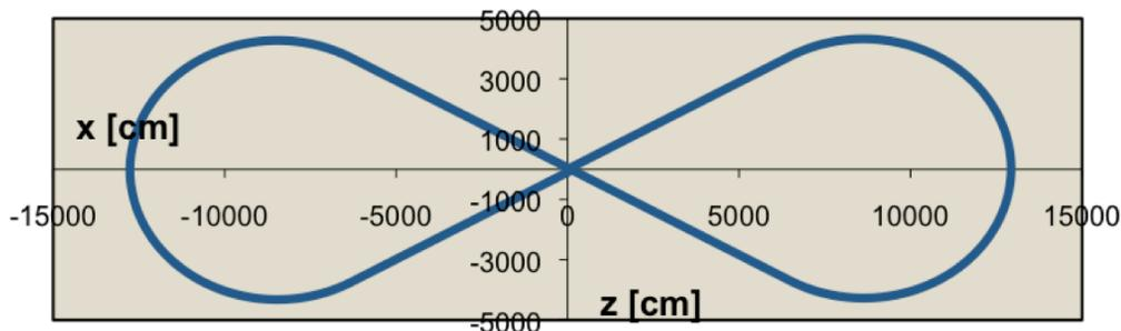
Figure 1: Footprint of figure-8 MEIC electron ring
