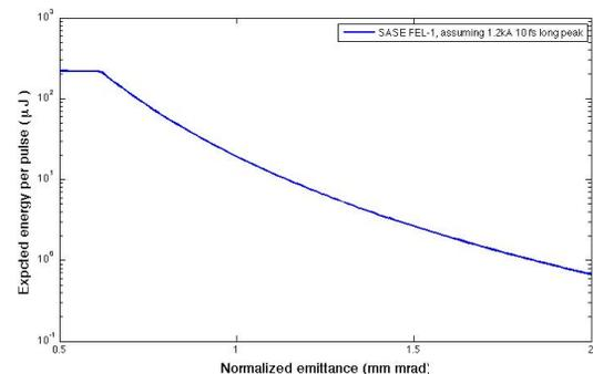
Figure 1: Expected energy per pulse as a function of emittance, in SASE configuration. The calculation relies on M. Xie's formula [8]. It is performed using six undulator sections and assuming a peak current of 1.5kA.
