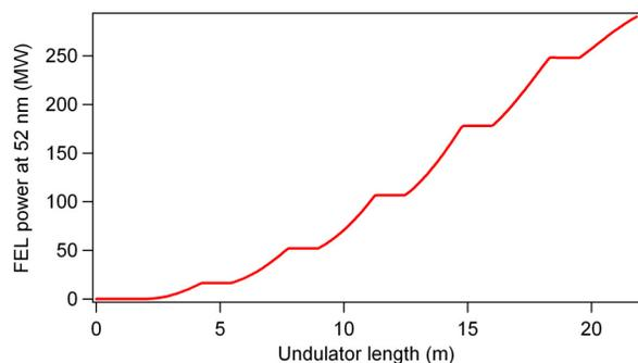
Figure 2: Predicted FEL power evolution at 52nm in the final radiator, in CHG configuration. The simulation is done with GINGER making use of an electron beam with an emittance of 1.5 mm mrad, energy spread 400 keV and peak current of 200 A.
