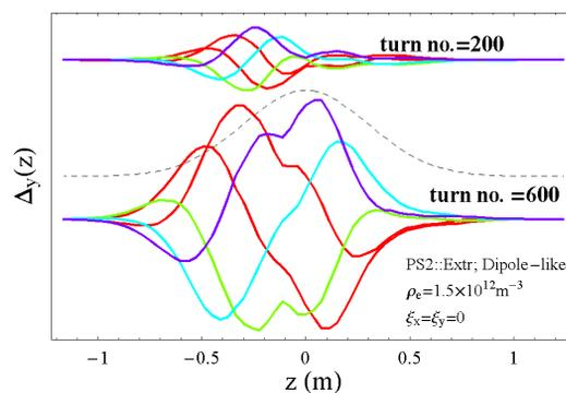
Figure 1: Beam vertical dipole moment monitored for 5 successive bunch passages starting from turn no. 200 and 600 above instability threshold. The dashed line represents the equilibrium bunch longitudinal profile. The beam head is at  $z > 0$ .
