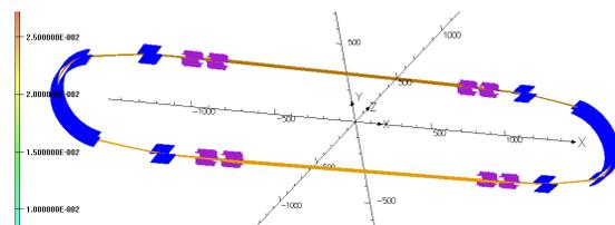
Figure 2: Model of the ELISA ring in OPERA3D. The Dimensions and distances were taken from [12]. All particles were tracked over 700 turns.
