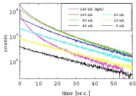
Figure 1: Decay of stored  $O^-$  beams at 22 keV [3].
