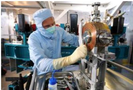
Figure 4: An EMMA RF cavity under test.
