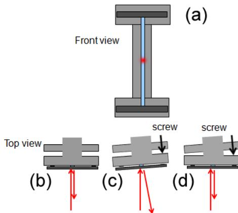
Figure 6: (a) sketch frontal view of a strip crystal mounted on its holder. (b-c-d) screw acting on the holder is used to compensate torsion; an optical setup acts as a feedback of the crystal alignment. See text for more details.
