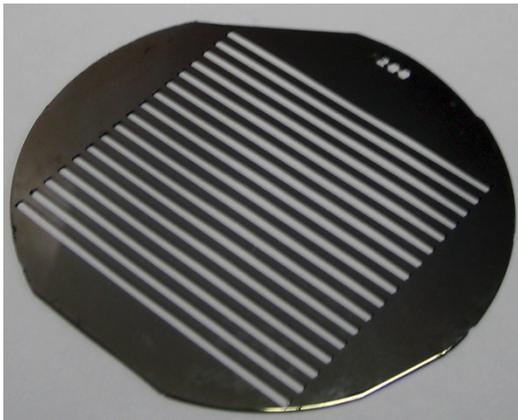
Figure 3: Si single crystal with equidistant rectangular slots obtained by anisotropic etching.
