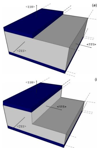
Figure 1: Schematic view of fabrication of a silicon crystal via anisotropic etching. (a) sample after patterning with  $\text{Si}_3\text{N}_4$  (dark regions) and prior to chemical attack; (b) the unmasked areas undergo etching along the  $\langle 110 \rangle$  direction while negligible erosion occurs along the  $\langle 111 \rangle$  direction. Proper timing allows one to make controlled indentations or complete cut of the sample.
