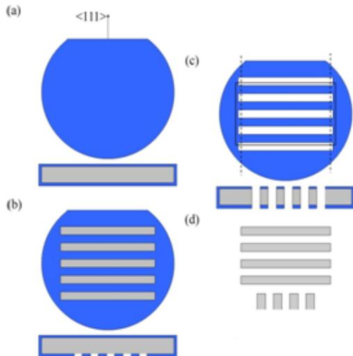
Figure 2: Fabrication of crystals for channeling (not to a scale) (a) deposition of a uniform 100-nm thick  $\text{Si}_3\text{N}_4$  layer, (b) patterning of  $\text{Si}_3\text{N}_4$ , (c) anisotropic KOH etching and mechanical dicing along either the dashed line to release a series of independent strip-like crystals or the solid line to manufacture a multi-strip crystal with a frame, (d) final removal of the  $\text{Si}_3\text{N}_4$  film.
