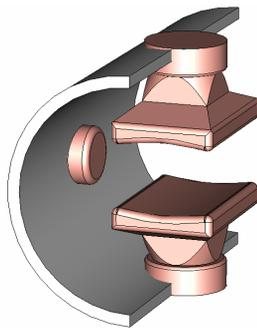
Figure 4: A proposed shape of the deflecting plates.
