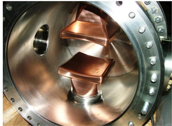
Figure 5: The prototype deflecting cell.
