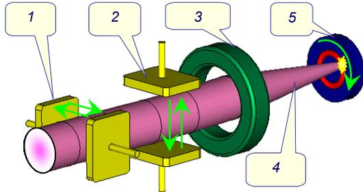
Figure 1: The general layout of the deflecting system.
