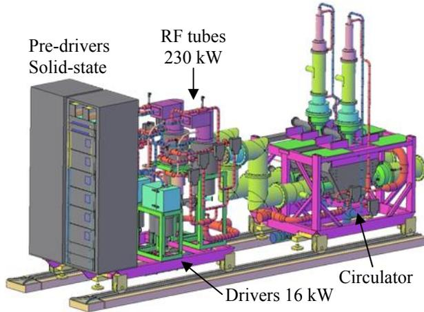
Figure 4: Schematic view of the RF power chain .
