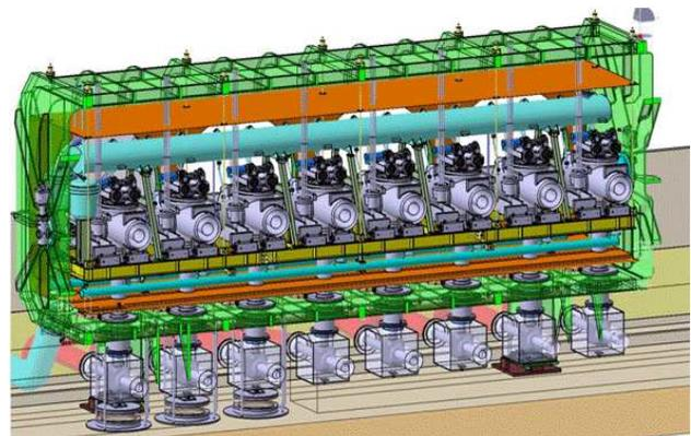
Figure 3: Overview of the EVEDA cryomodule.
