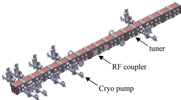
Figure 2: Schematic view of the RFQ with ports for cryo-pumps, tuners and RF coupler.
